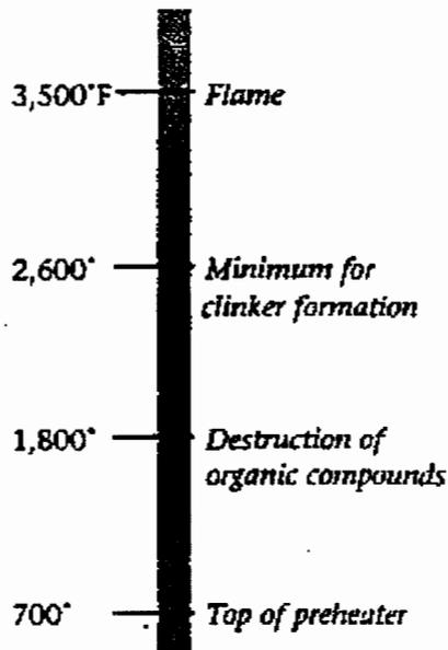
Figure 2 - Temperature Profile Preheater Dry Process Cement Kiln
