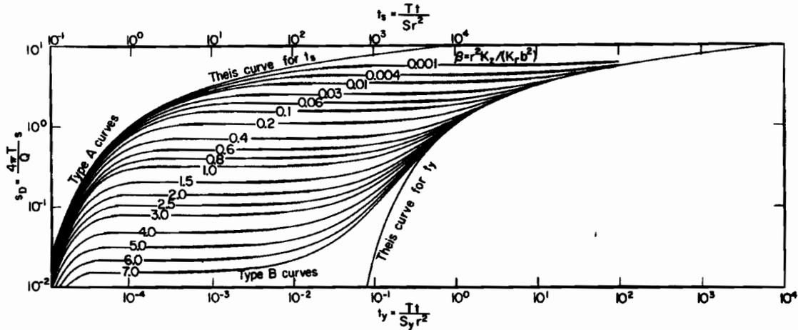
Fig. 1. Type curves for fully penetrating wells.
