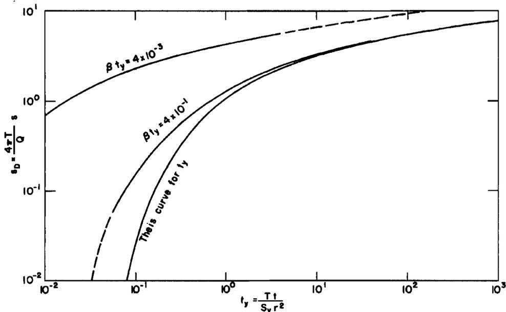
Fig. 4. Dimensionless distance-drawdown curves for fully penetrating wells at various values of  $\beta t_y = \text{const}$ .
