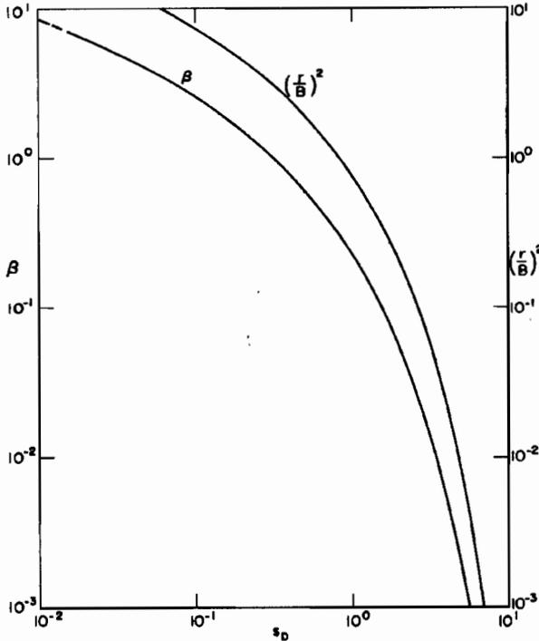
Fig. 5. Values of  $\beta$  and  $(r/B)^2$  versus  $s_D$  corresponding to horizontal portion of type curves for fully penetrating wells.
