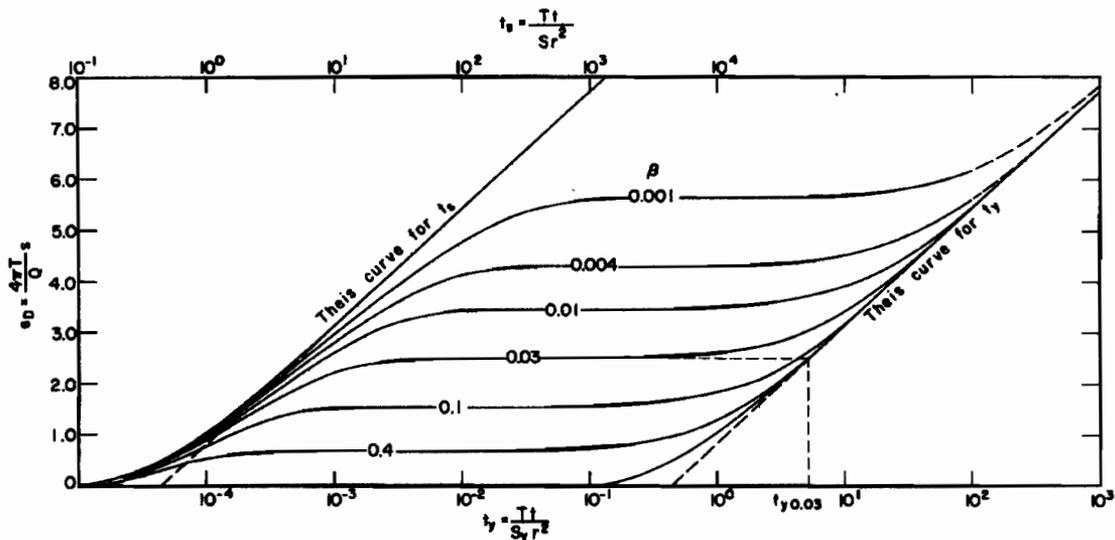
Fig. 2. Semilogarithmic relationship between dimensionless drawdown and dimensionless time in fully penetrating wells.
