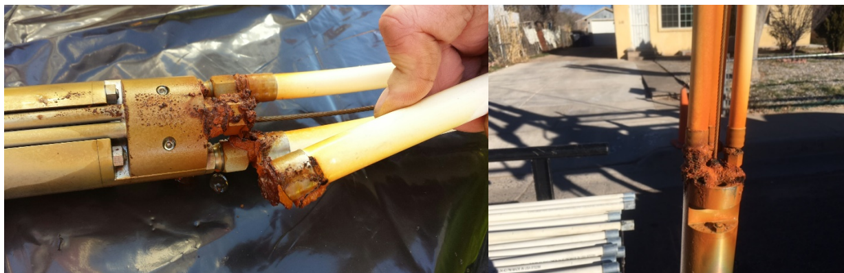
Figure 2. Pump pulled from well KAFB-106227 after approximately six months of deployment (left) with tubing fitting severed by corrosion. Pump pulled from KAFB-106208 after approximately three and a half years of deployment (right).
