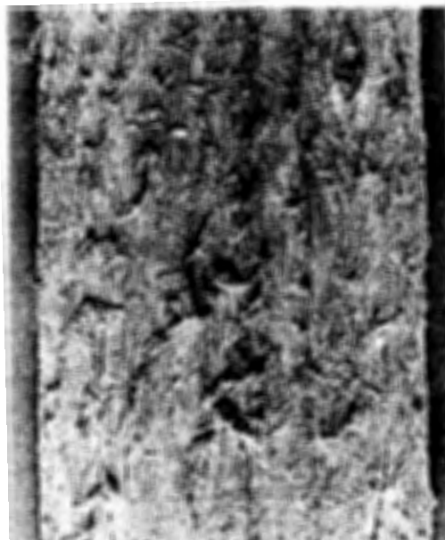
Figure 39-3 • Fibrillated Wood—Caused by Chemical Attack
