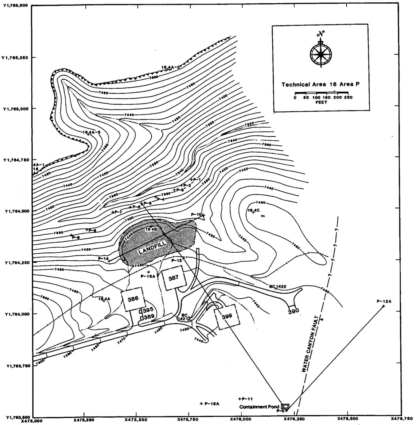
Figure 2. Site map of Technical Area 16, Area P. Boreholes are marked with crosses, numbered P-0 through P-16A. Additional crosses are surveyor's marks.
