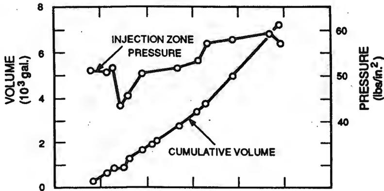
Fig. 4. Injection rate, injection-zone pressure, and cumulative volume of water injected into tuff during test 3 at site 1, May 19-21, 1965.
