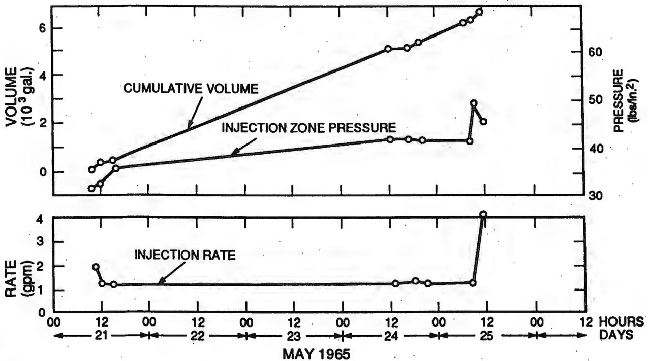
Fig. 5. Injection rate, injection-zone pressure, and cumulative volume of water injected into tuff during test 4 at site 1, May 21-25, 1965.
