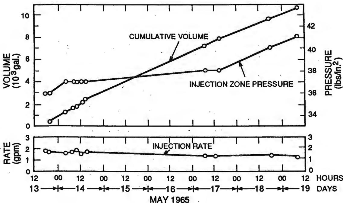
Fig. 3. Injection rate, injection-zone pressure, and cumulative volume of water injected into tuff during test 2 at site 1, May 13-19, 1965.
