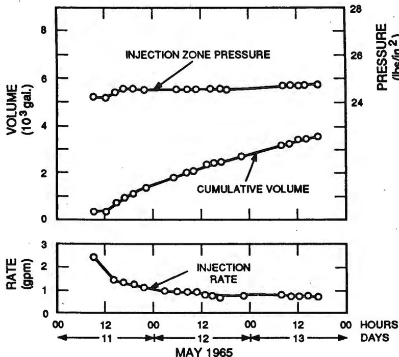
Fig. 2. Injection rate, injection-zone pressure, and cumulative volume of water injected into tuff during test 1 at site 1, May 11-13, 1965.
