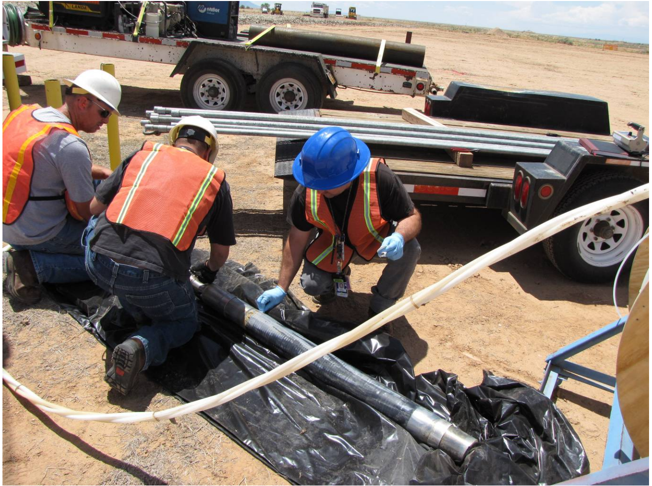
Figure 2-2 Screening the MWL-MW4 packer for radiological contamination by an RCT, May 27, 2009. View to the south.
