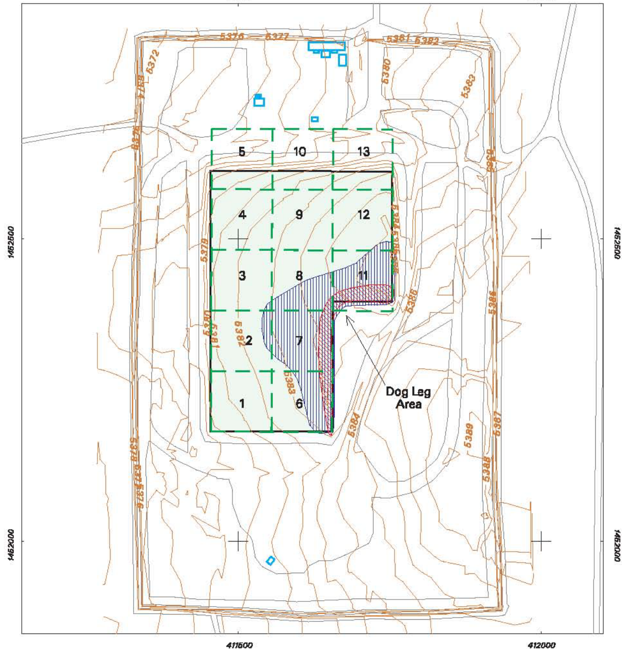
Figure 19 Mixed Waste Landfill Cover Grid Blocks and Locations of Native Soil Layer Wedge Lifts 1 & 2
