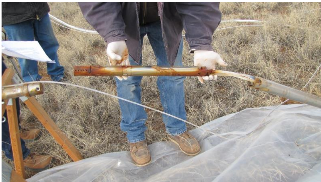
Figure 4-4. Photograph of the Stainless Steel Bennett™ Sampling Pump After Removal from MWL-MW4 on December 16, 2014 Showing Substantial Corrosion
