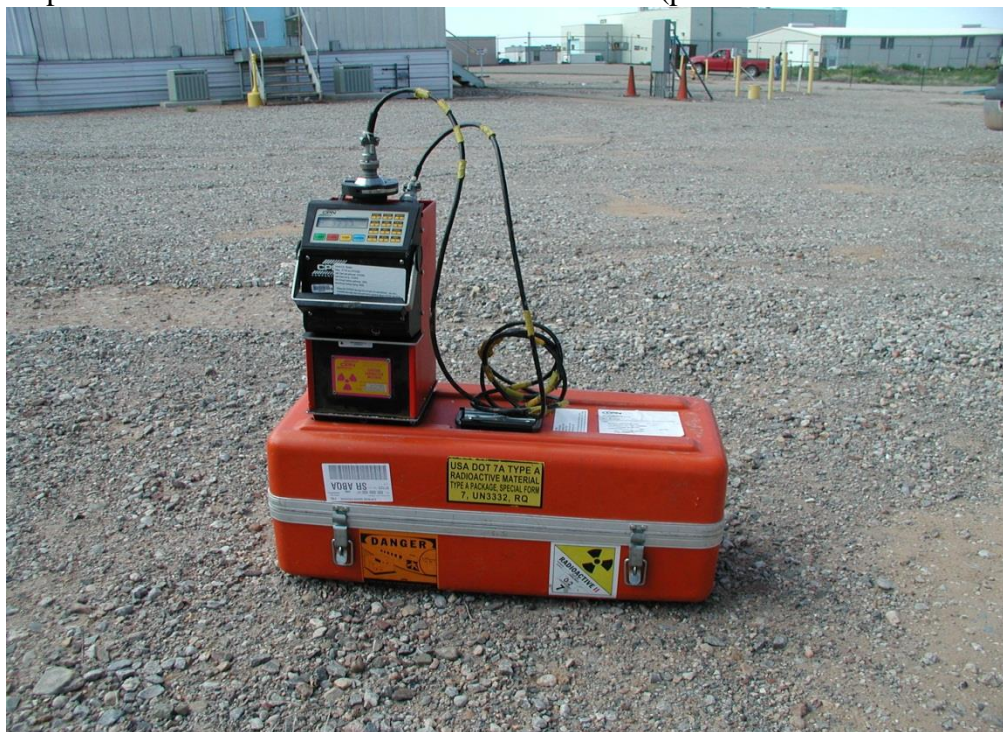
CPN probe/shielded control box and instrument case (probe contained in shielding)
