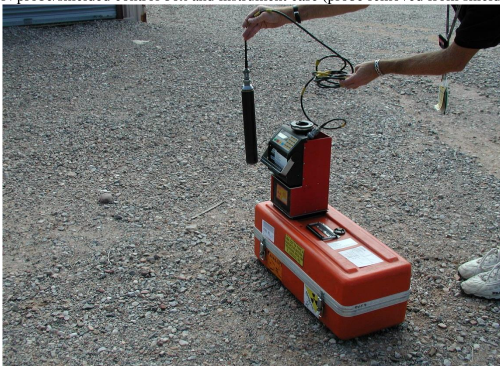
CPN probe/shielded control box and instrument case (probe removed from shielding)
