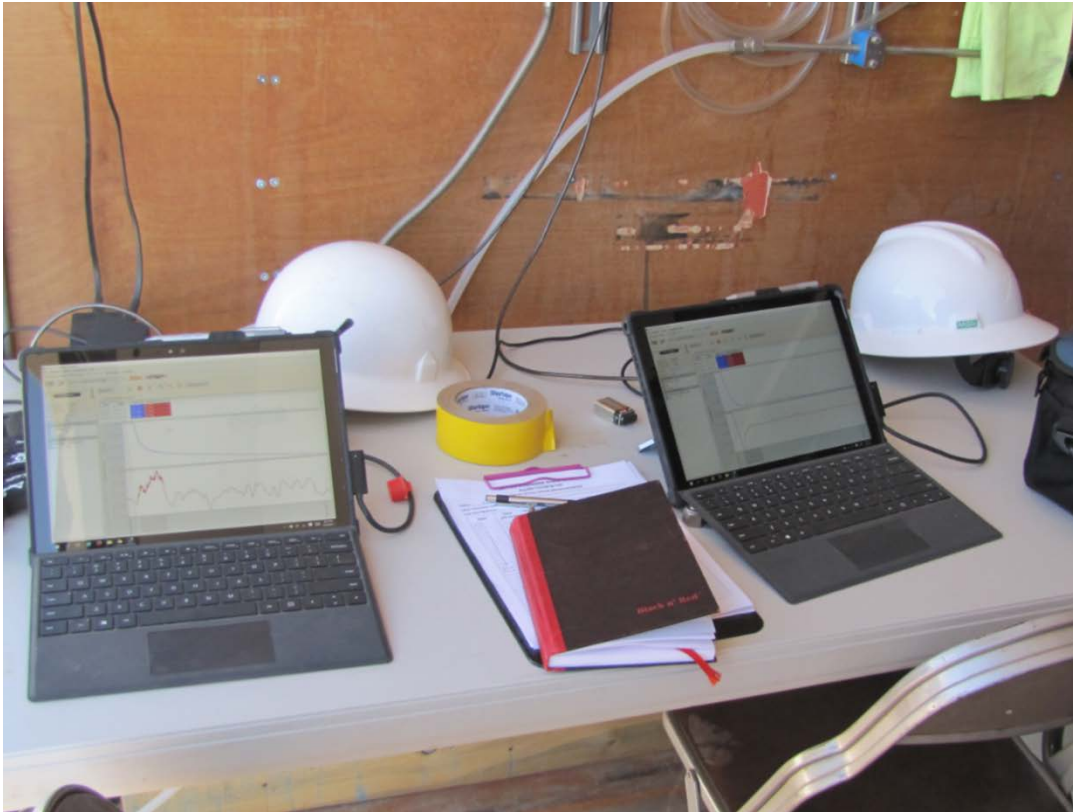
View to the East. Detail of Laptop Computer Setup inside the Sampling Truck for Real-Time Viewing of Water Level Data from Burn Site Well and CYN-MW11 Transducers.
