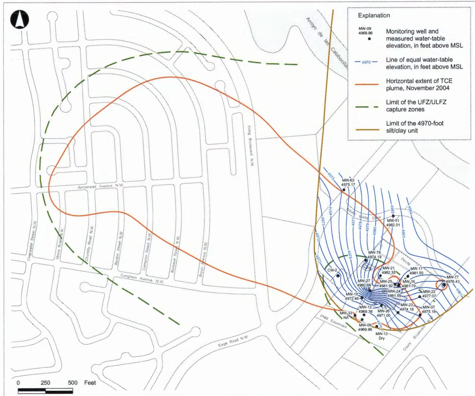
Figure 5.10 Elevation of the On-Site Water Table - November 1, 2005
