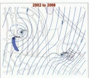
Reverse Particle Tracking Results during CW-1 and CW-2 Pumping with Average Water Levels 2002-2008
