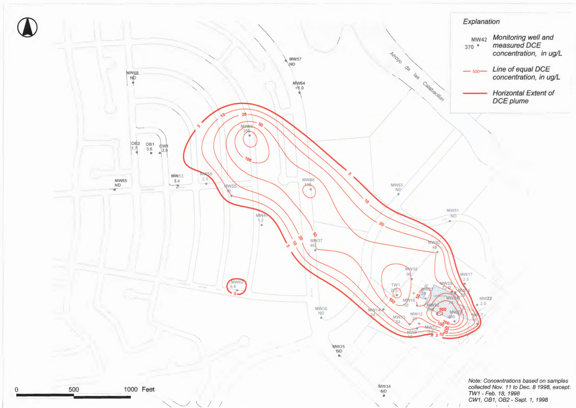
Figure 2.16 Horizontal Extent of DCE Plume - November 1998
