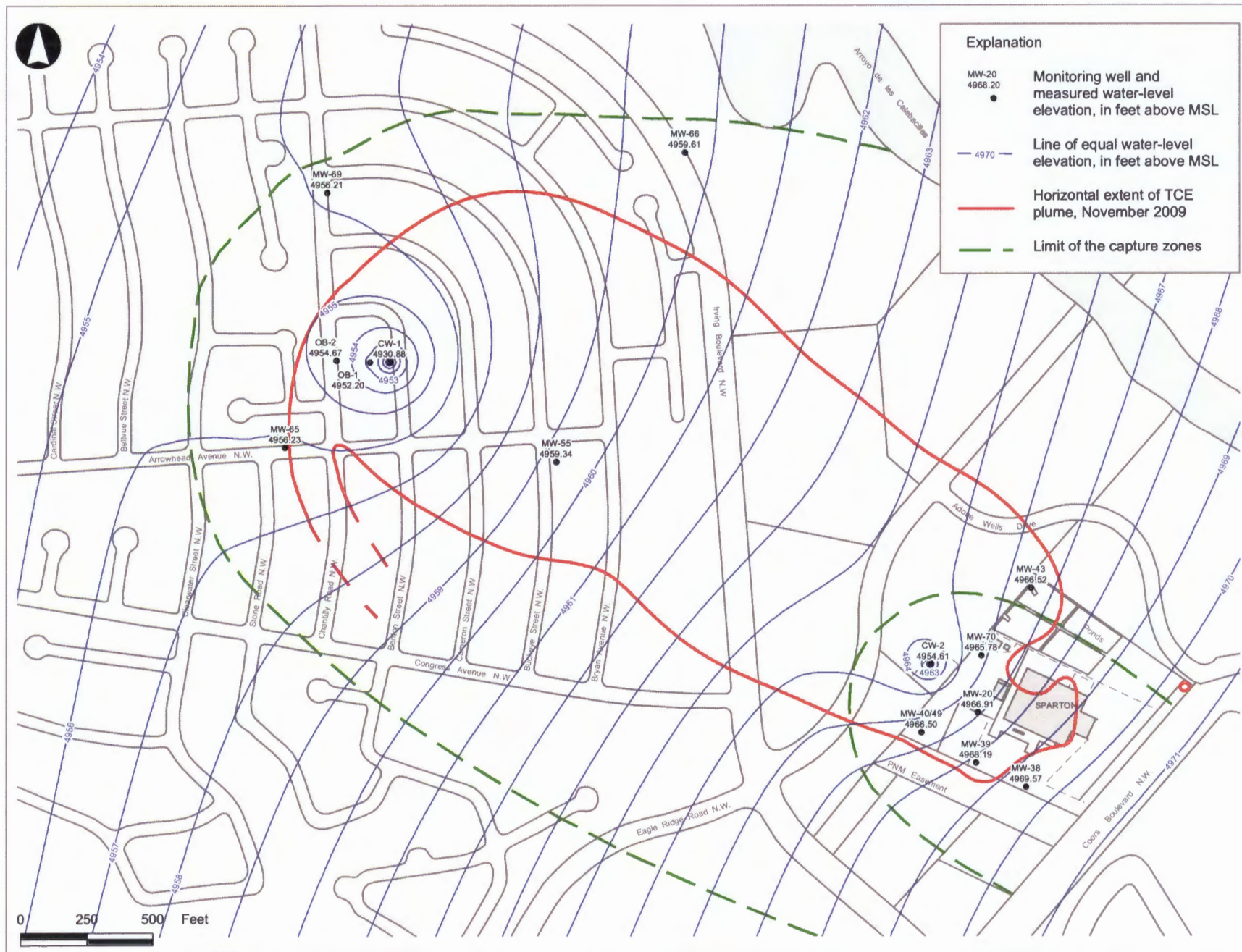
Figure 5.3 Elevation of Water Levels and Limits of Containment Well Capture Zones in the LLFZ - February 9-10, 2010
