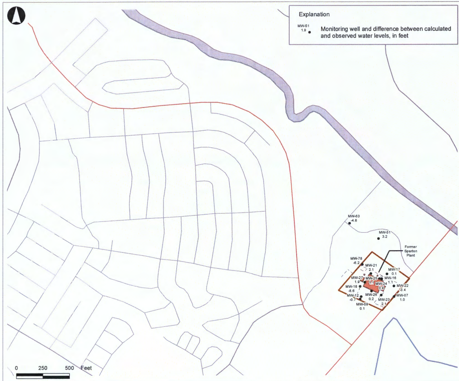
Figure D.4 Residuals between Observed and Calculated 2010 Water Levels in On-Site UFZ Wells
