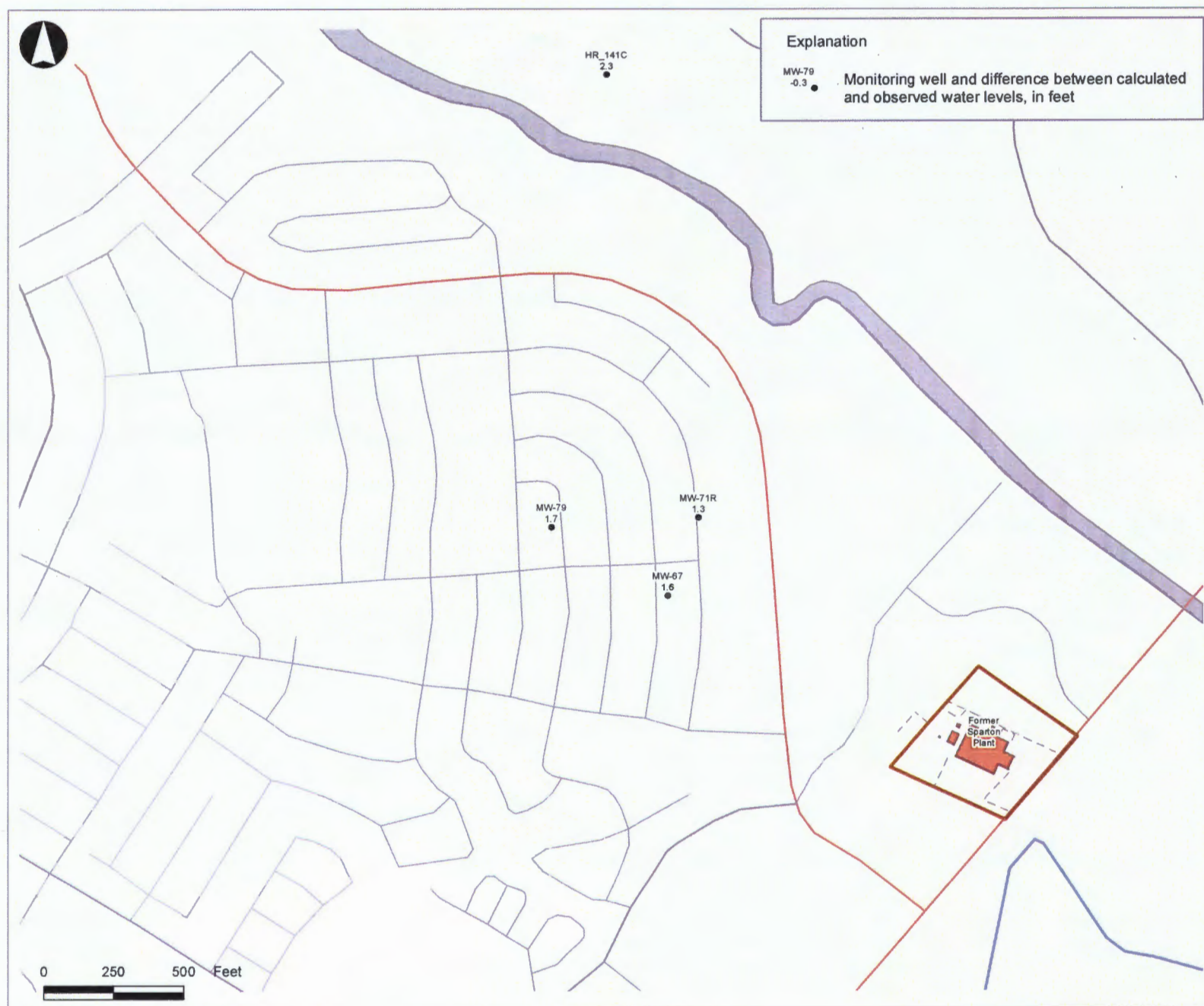
Figure D.6 Residuals between Observed and Calculated 2010 Water Levels in DFZ Wells
