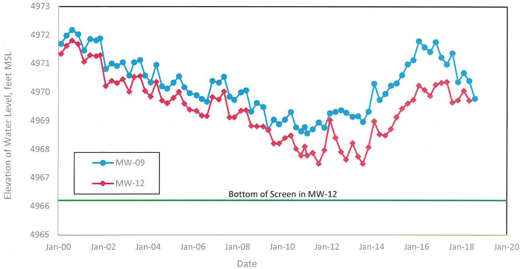
**Figure 2 - Comparison of Hydrographs of Monitoring Wells MW-09 and MW-12**
