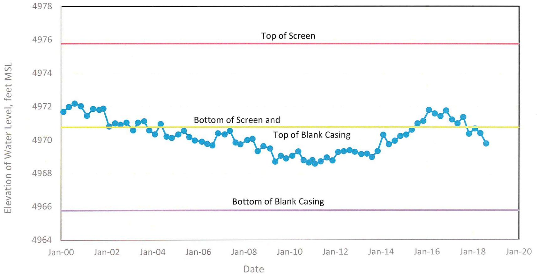
**Figure 1 - Hydrograph of Monitoring Well MW-09**
