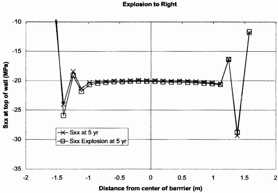
**Figure 2-2 Vertical (Radial) Stress Profile at Top of Block Wall During an Explosion Occurring 5 Years after Emplacement**
