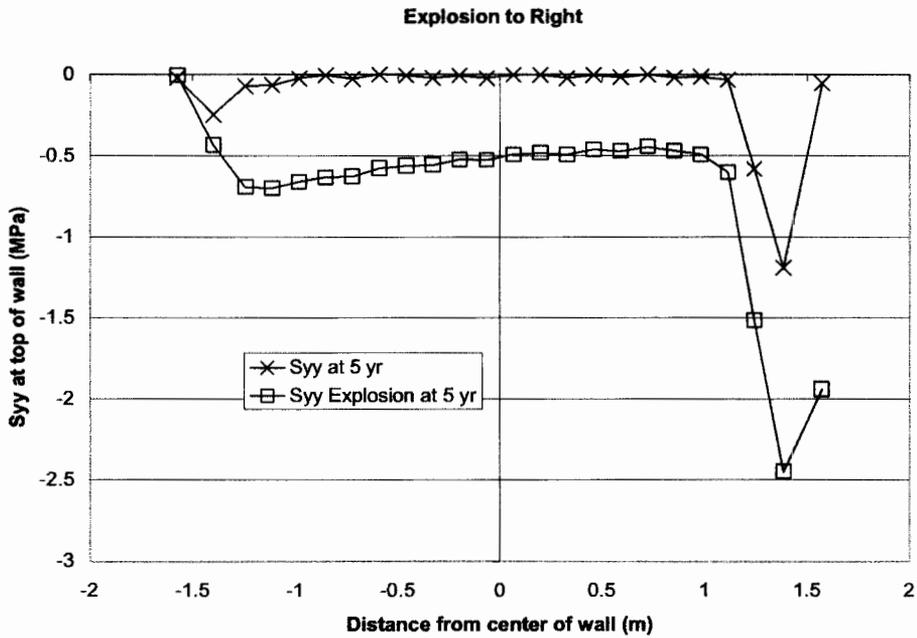
**Figure 2-3 Horizontal (Axial) Stress Profile at Top of Block Wall During an Explosion Occurring 5 Years after Emplacement**
