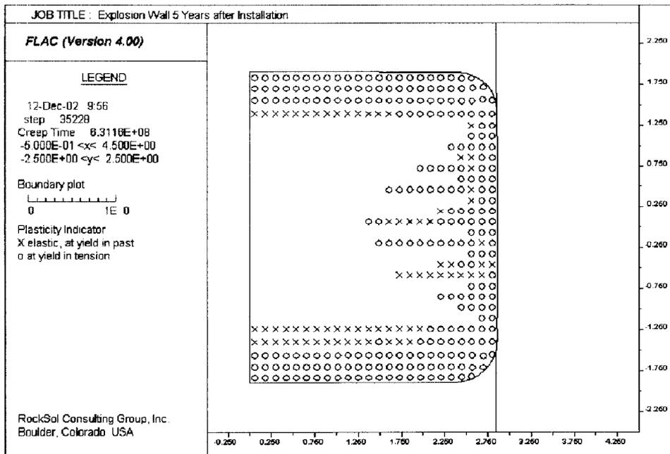
**Figure 2-6 Plasticity State in Block Wall at 5 Years**
