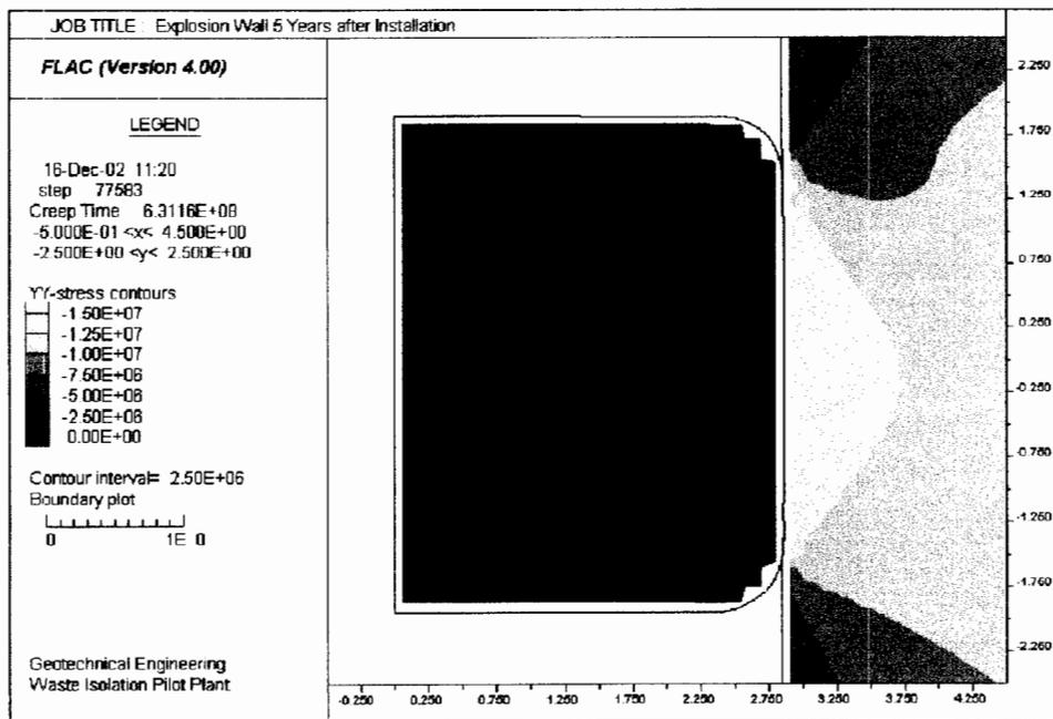
**Figure 2-5 Horizontal (Axial) Stress Contours in Block Wall During an Explosion Occurring 5 Years after Emplacement**
