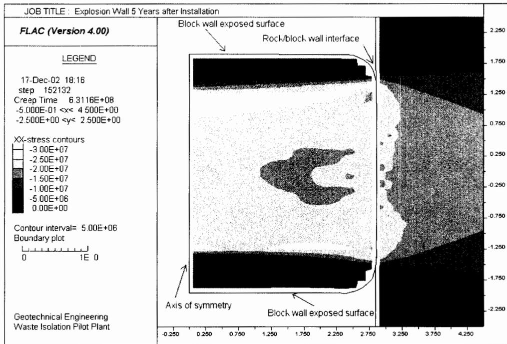
Figure 2-4 Vertical (Radial) Stress Contours in Block Wall During an Explosion Occurring 5 Years after Emplacement
