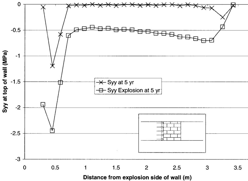
**Figure 2-3 Horizontal (Axial) Stress Profile at Top of Block Wall During an Explosion Occurring 5 Years after Emplacement**
