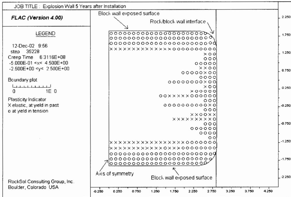
**Figure 2-6 Plasticity State in Block Wall at 5 Years Without Explosion**
