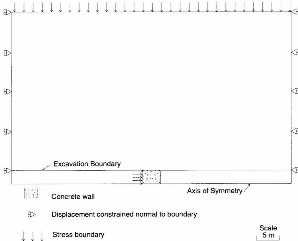
**Figure 2-1 Creep Plus Explosion Model Geometry and Boundary Conditions.**
