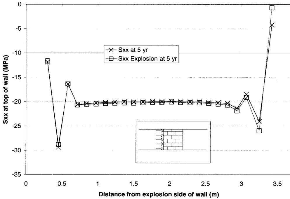
**Figure 2-2 Vertical (Radial) Stress Profile at Top of Block Wall During an Explosion Occurring 5 Years after Emplacement**
