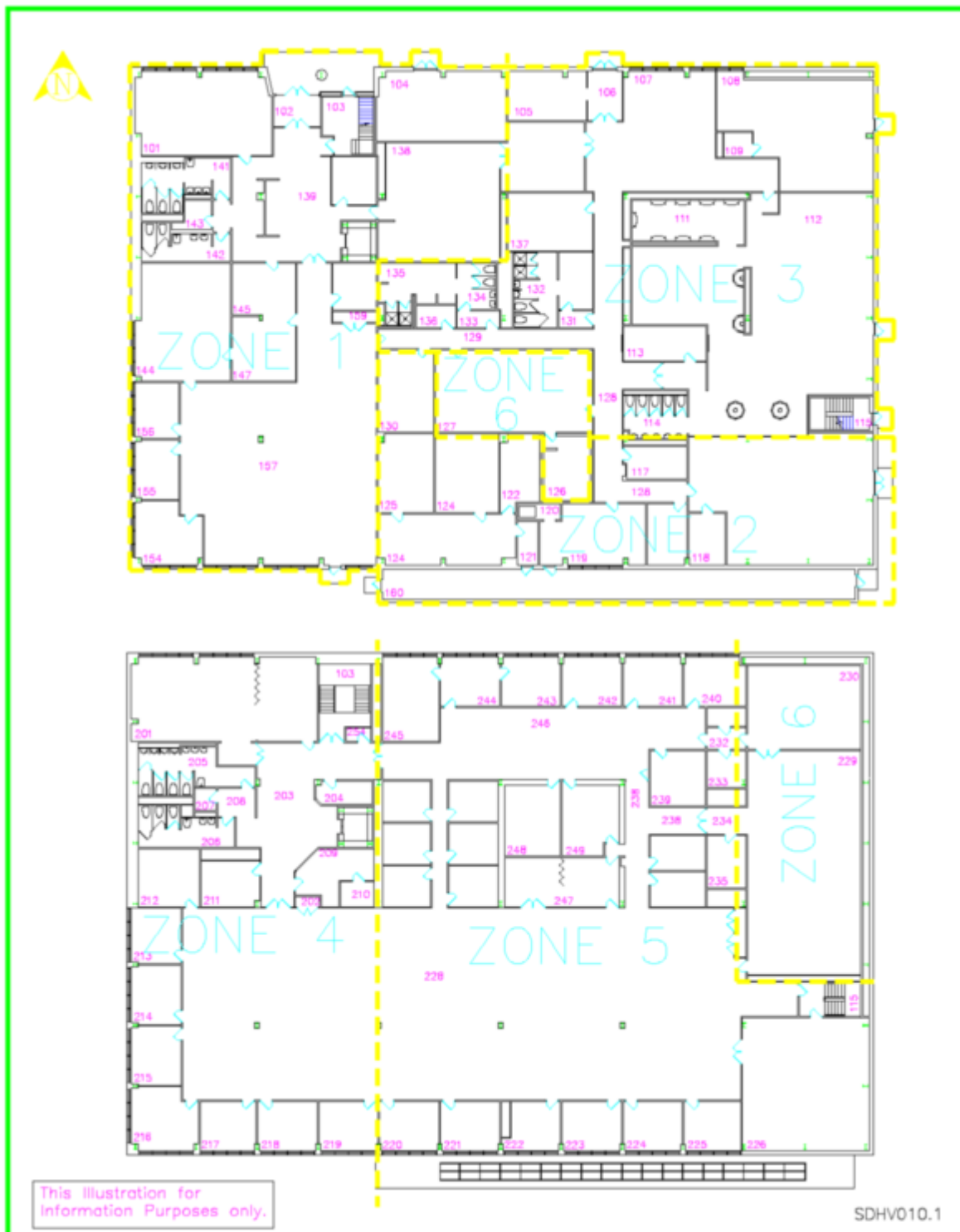
FIGURE HV III-1: HV03 Zone Boundaries for Support Building HVAC
