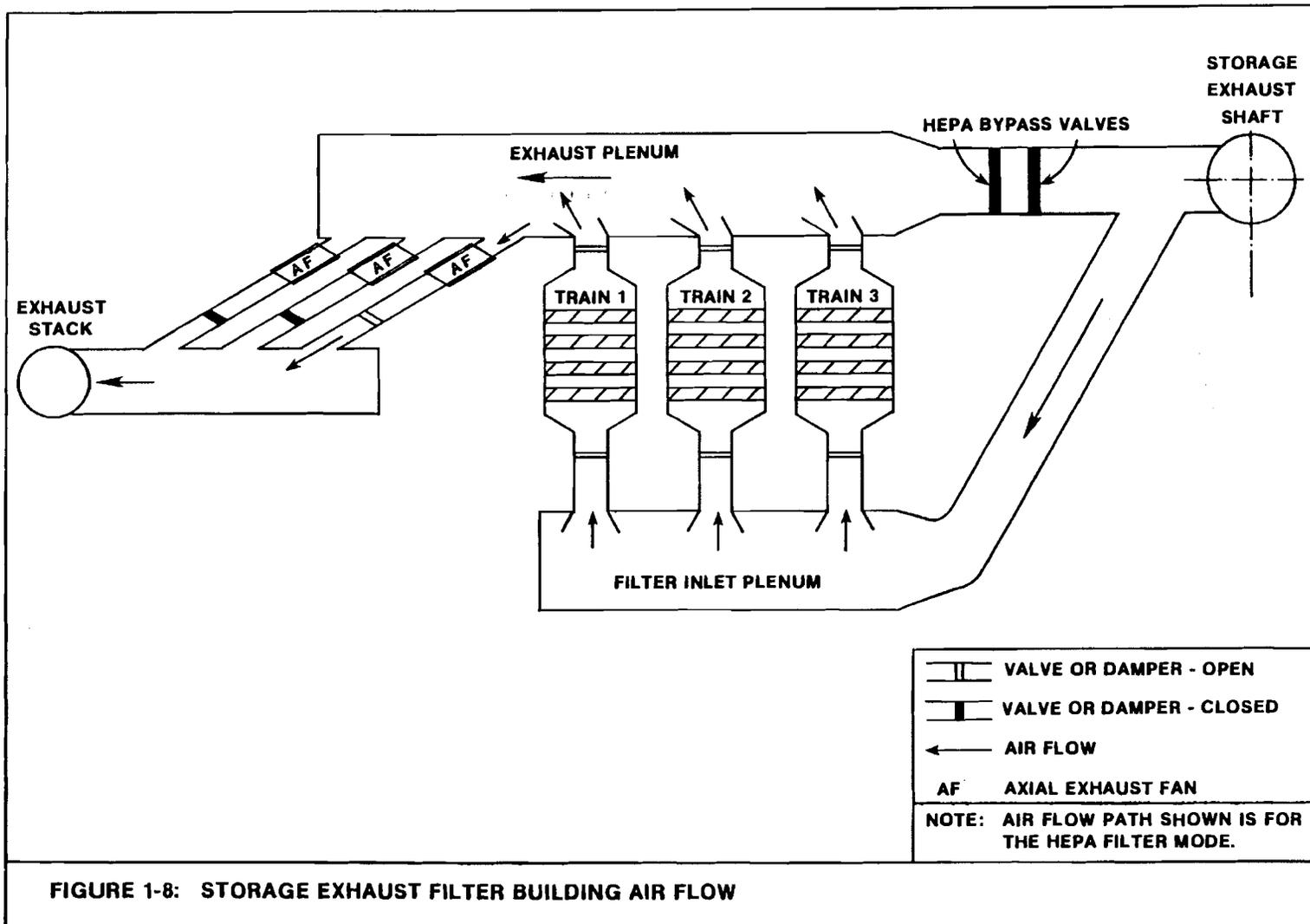
**FIGURE 1-8: STORAGE EXHAUST FILTER BUILDING AIR FLOW**
