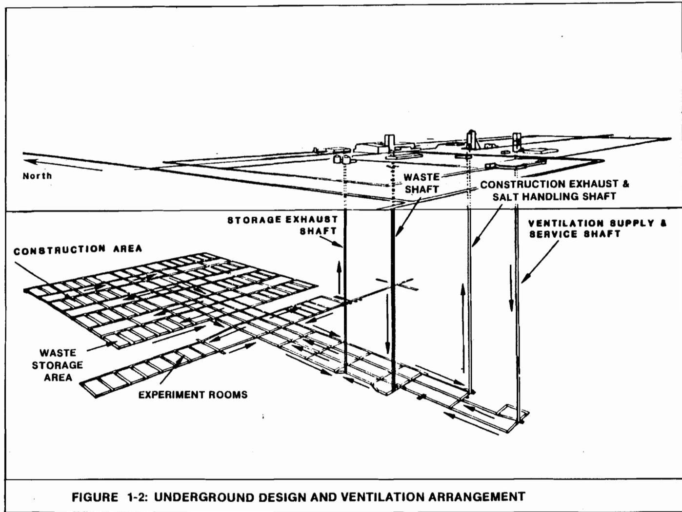
The Construction Exhaust and Salt Handling Shaft will be used to bring mined rock to the surface and to exhaust air from the mining operations area. The Storage Exhaust Shaft will exhaust air from the underground storage areas to the Storage Exhaust Filtration Building.
