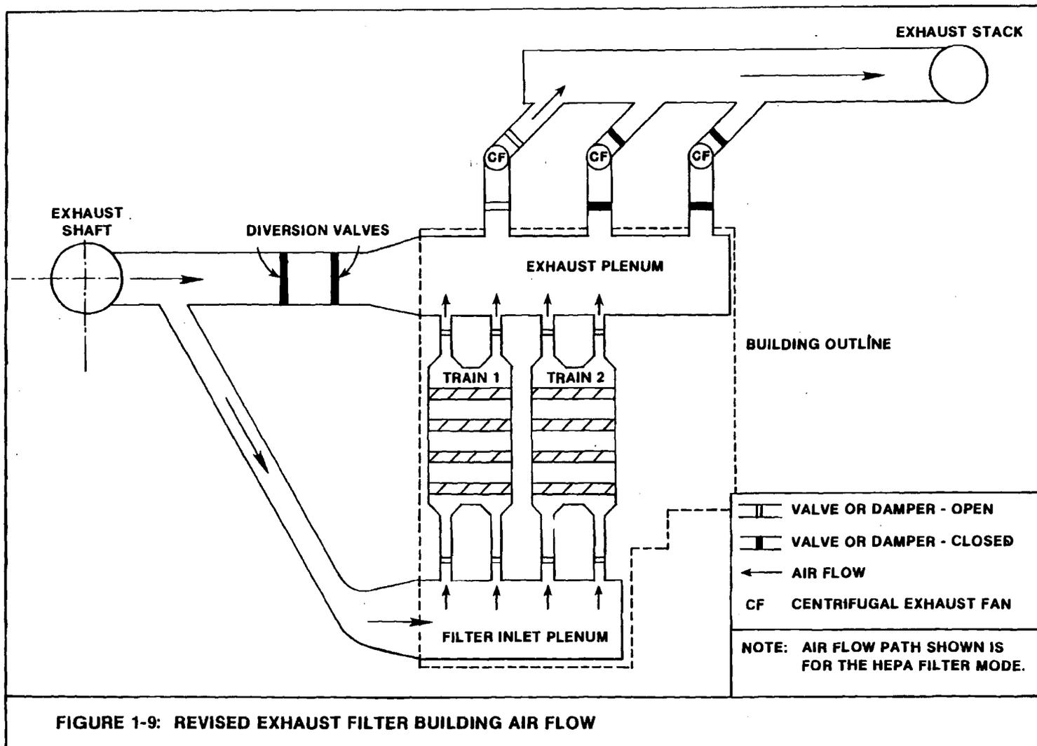
**FIGURE 1-9: REVISED EXHAUST FILTER BUILDING AIR FLOW**
