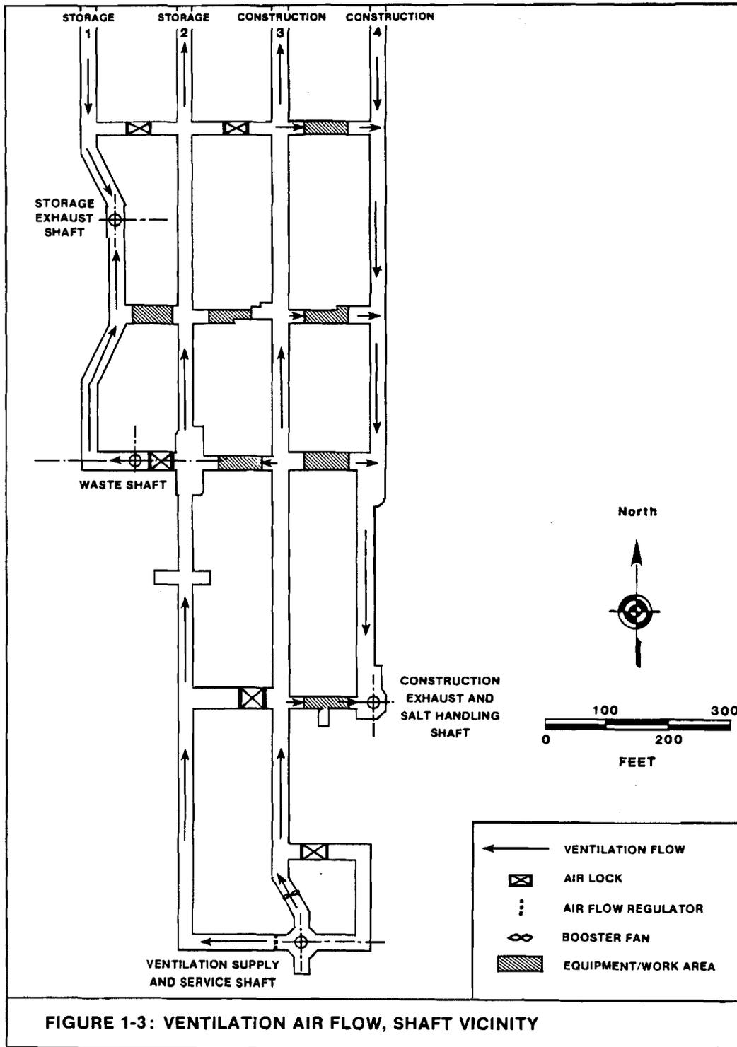
FIGURE 1-3: VENTILATION AIR FLOW, SHAFT VICINITY
