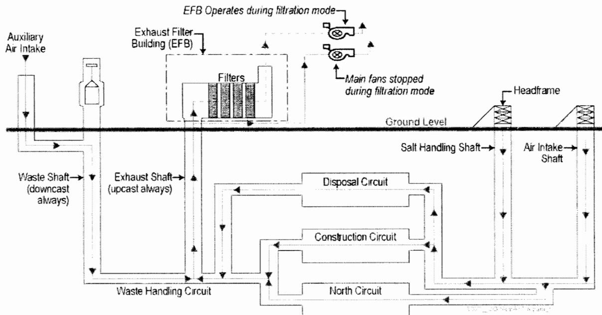
**Figure 3. WIPP Ventilation System Serving the Underground—Current Configuration**
