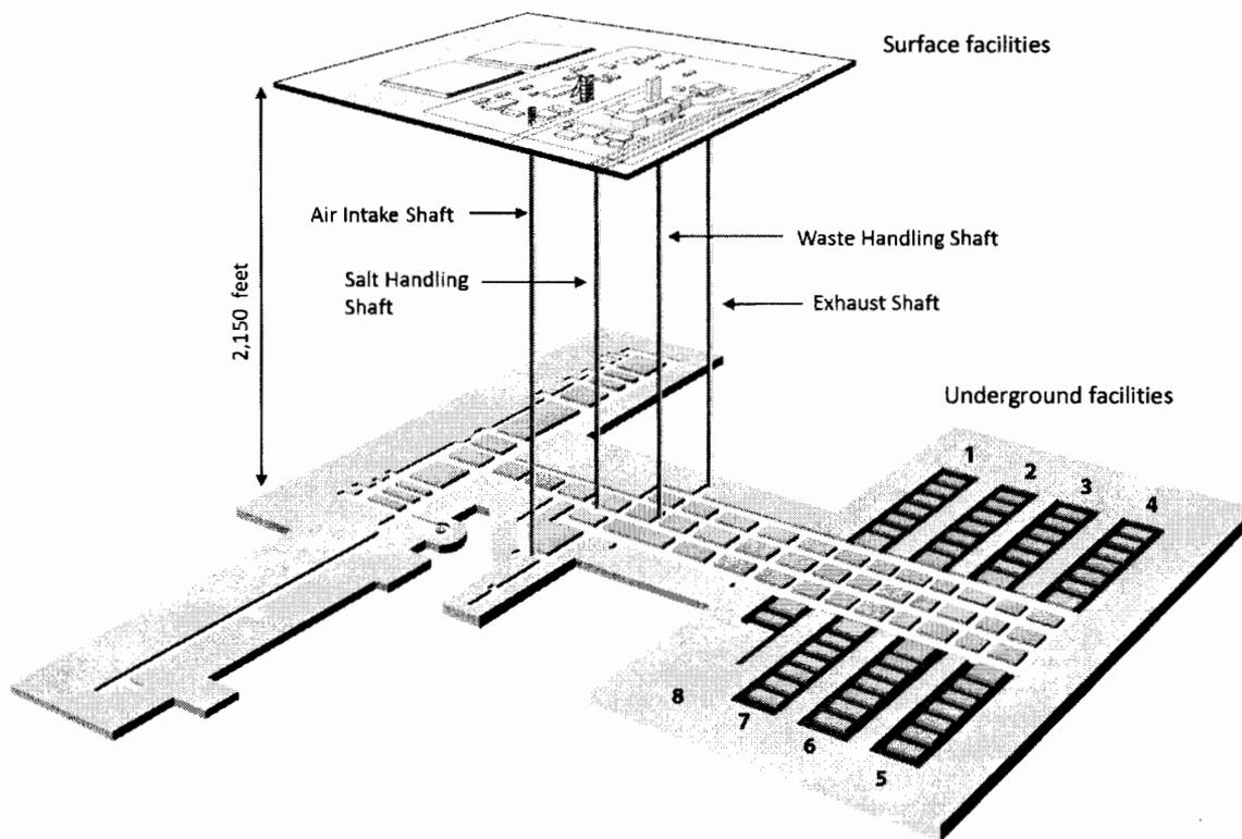
**Figure 1. WIPP Surface, Shafts, and Underground Facilities**
