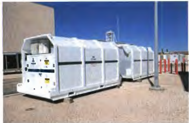
Safe havens provide life-saving shelter for underground workers in the event of an emergency.
