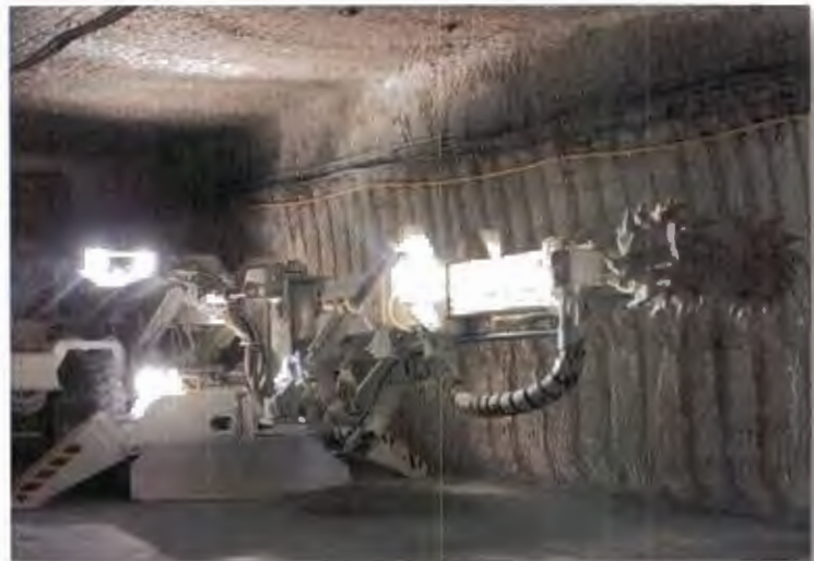
Miners operating seal cutters are well away from the location where the rock is being removed.
