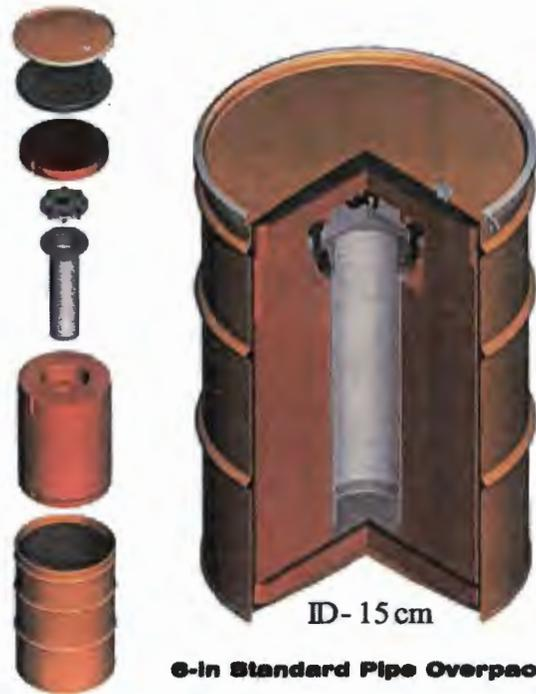
Primarily used for shipping larger amounts of fissile material (<200g)
