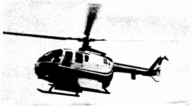
FIGURE 2. MBB BO-105 HELICOPTER WITH DETECTOR PODS
