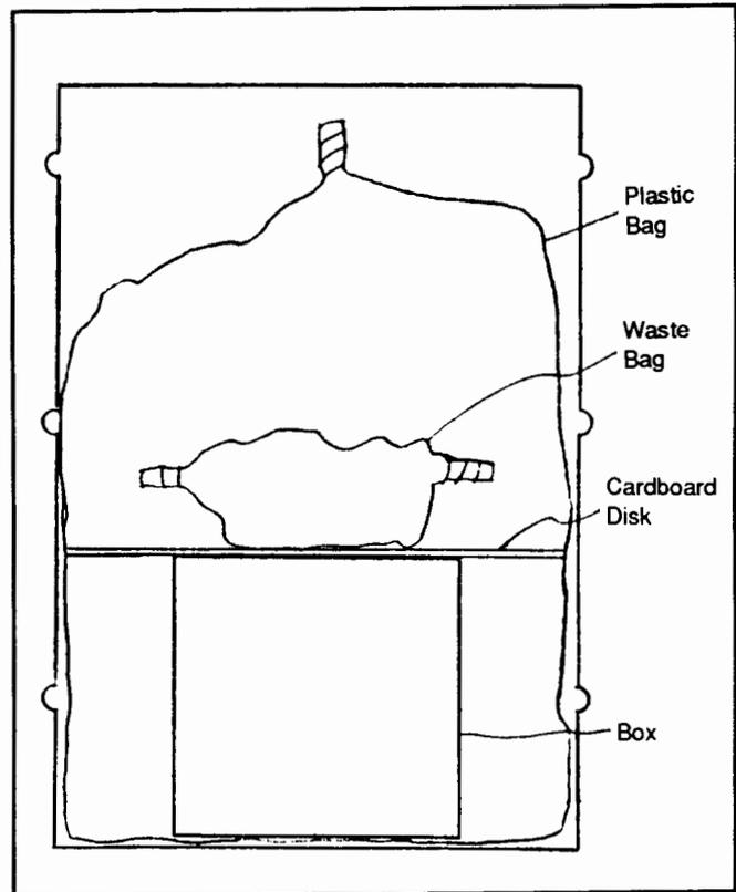
FIGURE 5. Specially Prepared 55-Gallon Drum
