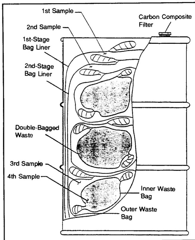
FIGURE 3. Sectioned Combustible Waste Drum
