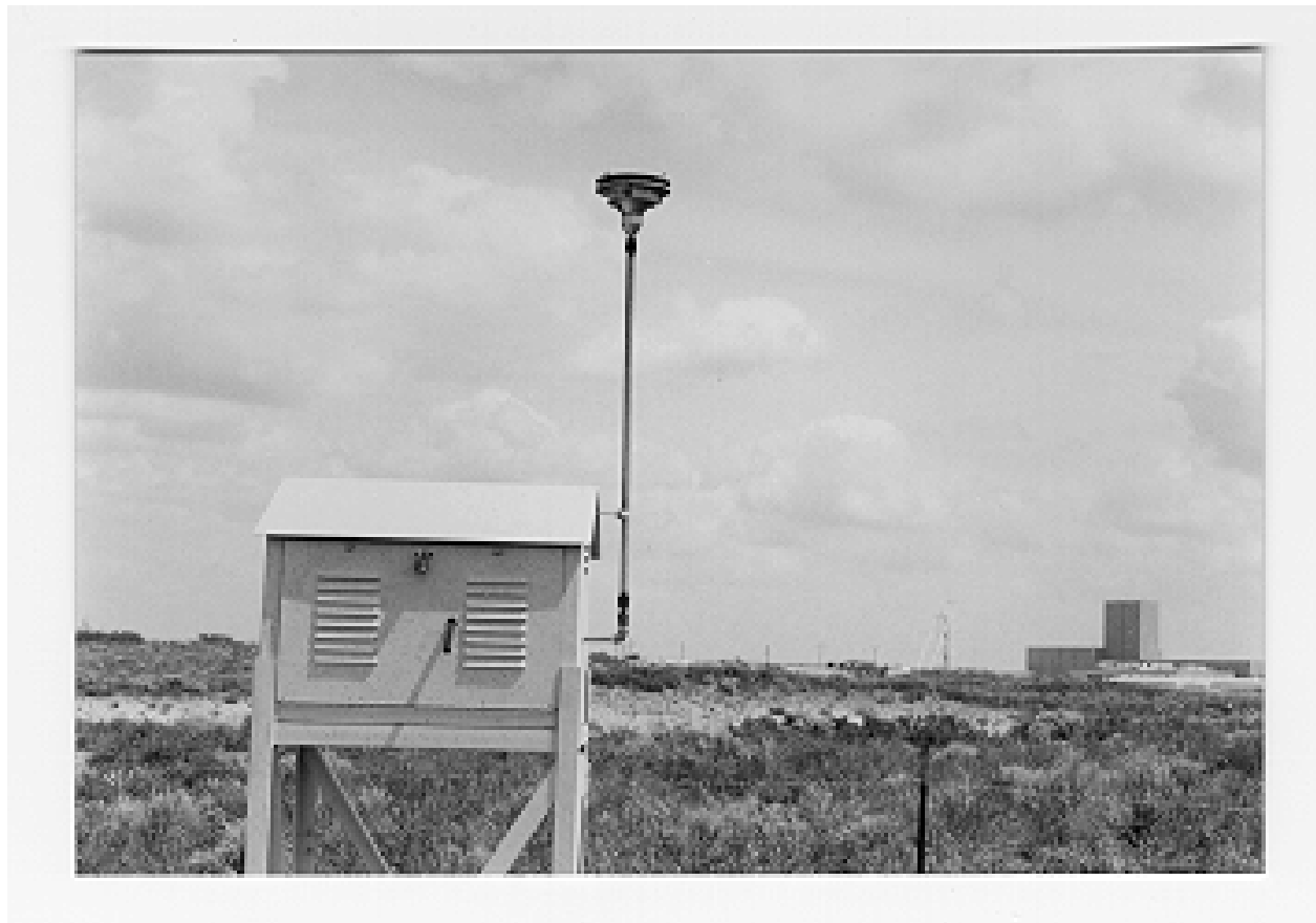
Figure 7. Typical EEG WIPP Site Low Volume Air Sampling Station
